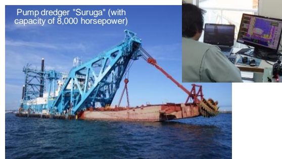
Checking the dredging status with GNSS and a tidal level observation system
