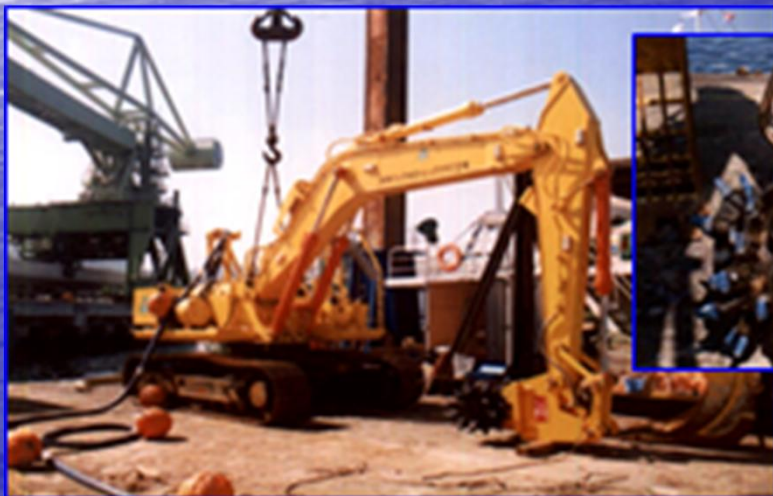
ツインヘッダ Twin header (固結粘土の掘削) (Excavating consolidated clay)
