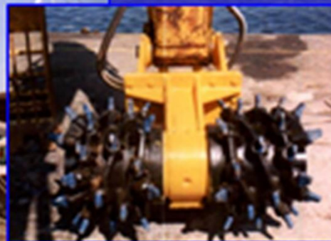
ツインヘッダ Twin header (固結粘土の掘削) (Excavating consolidated clay)
